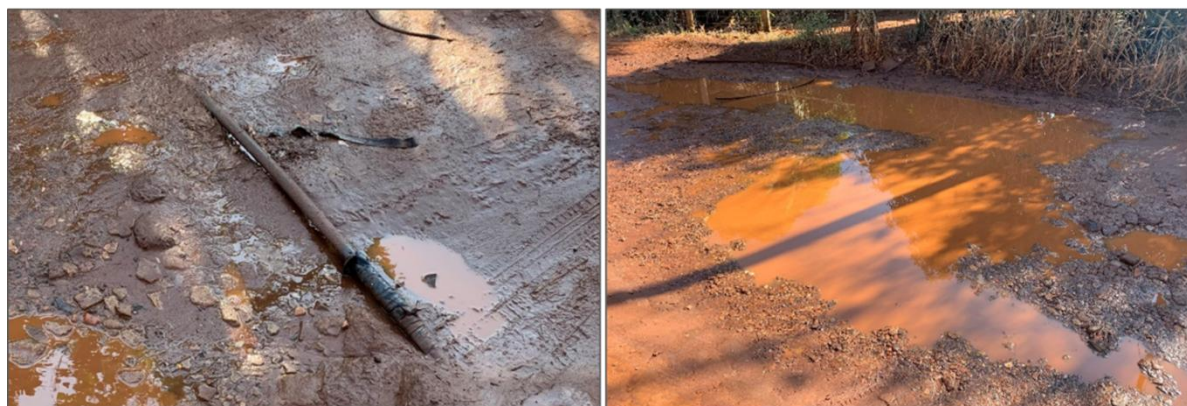
FIGURE 3 IMAGES OF POLYETHYLENE HOSES AND LEAKS IN THE FAZENDA DA BARRA SETTLEMENTS, RIBEIRÃO PRETO, SÃO PAULO, BRAZIL, 2024
